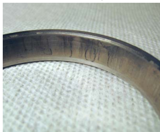
Figure 2: Pitted bearing race
