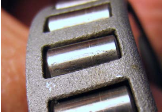
Figure 3: Pitted bearing roller
